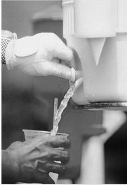
to use, the operator reverse-fills an empty, one-use plastic liner with water. The system is completely sealed from any outside elements, including ice, until the water reaches the drinking cup.
